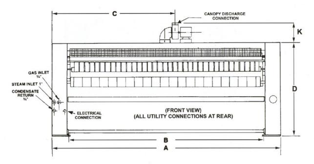
Allow minimum of 18" (457 mm) clearance at ends of machine for maintenance access. Canopy blower requires 10" diameter venting; 1050 CFM. Provide adequate make-up air according to current local requirements. Canopy vent must be independently discharged to atmosphere. Do not interconnect with other vent lines. Do not use for construction purposes unless certified correct by CMV Sharper Finish, Inc. Also available 85", 90", 100", 110", or 132".
