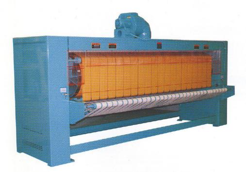
Convenient discharge height. Finished work delivered to the rear of the machine is raised to a height of over 32" inches (815 mm) by an angled conveyor. This increased height allows this machine to be used with all automatic folding machines. In addition, if work is to be hand folded the increased height increases productivity and reduces operator fatigue.
